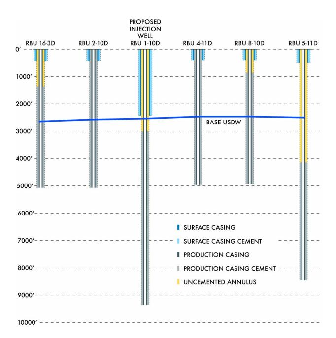
While Class II rules do not explicitly require surface casing to extend below the base of the lowest USDW,<sup>6</sup> they do require that, "all Class II wells shall be cased and cemented to prevent movement of fluids into or between underground sources of drinking water,"<sup>7</sup> and that the depth to the bottom of all USDWs be considered in determining and specifying casing and cementing requirements.<sup>8</sup>
